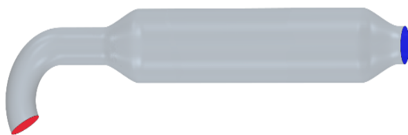
Fig. 4. Geometric representation of the CFD model developed for the plasma-arc furnace reactor quench probe.
